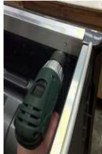
18. To fit the tailgate profile, measure and mark the centre of the tailgate and the aluminium profile.
