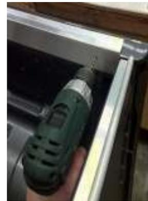
6. To fit the tailgate profile, measure and mark the centre of the tailgate and the aluminium profile. Remove the red backing tape from the underside of the profile. Press the profile down the inside face of the tailgate to align the two centre marks keeping the taped surface square with the top edge of the tailgate. Using the PVC drill template locate the templates along the bottom edge of alloy, mark the locations onto alloy. With a 4mm drill bit, drill and rivet each of the 3 marked holes.
