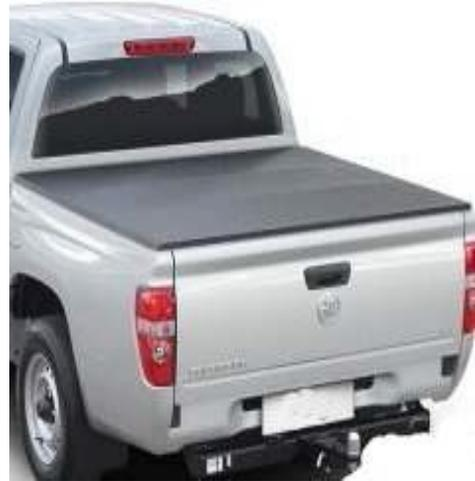
**You can adjust your tonneau, to make it tighter or looser, by simply raising or lowering the height of your tonneau support bar**
