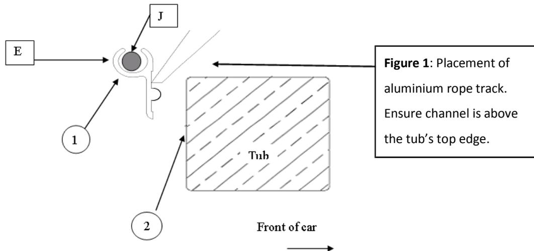
3. Using a 4 mm drill bit, drill 6 holes 50mm from the end of each of the aluminium rope tracks into the front of tub.
