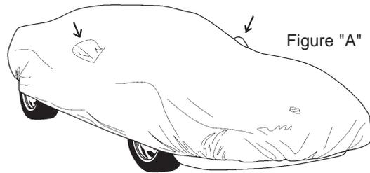
Some vehicles have very sharp bumpers, hood ornaments, moldings, etc. We recommend that you reinforce the inside of the cover at areas exposed to severe abrasion, using cloth-reinforced duct tape or vinyl tape which may be purchased at hardware, plumbing or automotive stores. This will help extend the use of your cover.
